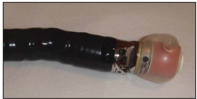
Fig 2. — High-frequency ultrasound waves are transmitted from the transducer at the tip of the echoendoscope to the target tissue. For optimal imaging, a balloon surrounding the transducer is inflated with water to improve ultrasound transmission.
